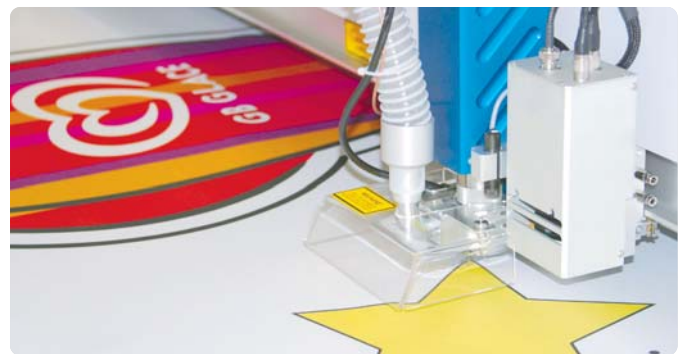
Lasercutting of printed materials by camera recognition
